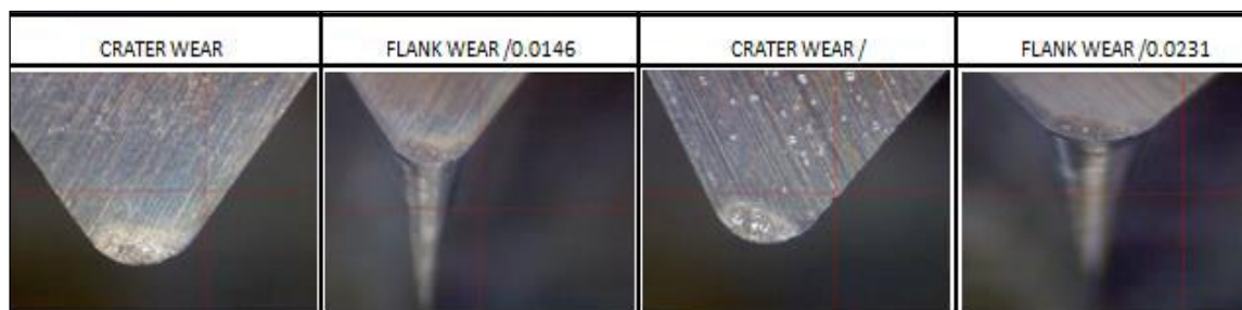
Fig.5. Cutting tool images obtained from RAPID I Machine
